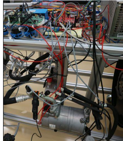
Figure 5 Heat pump test bench: (left) first measurements; (right) test bench photo
