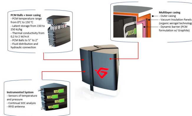
Figure 1: Example of thermal energy storage subsystem with PCMs and VIPs materials implementation
